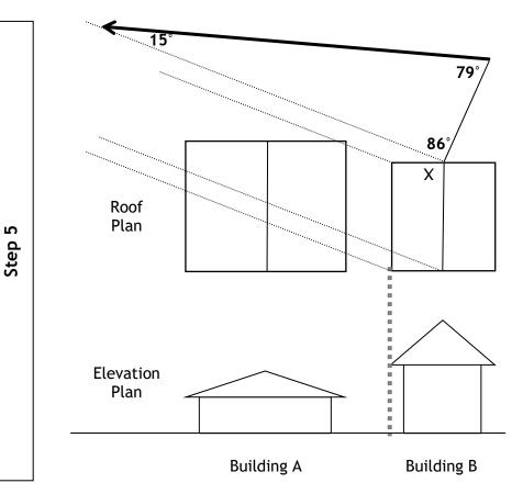
5. Draw a 79° angle from the end of Segment B. Find the point which this new line intersects the shadow line. This creates a 15° angle - the altitude angle of the sun.
