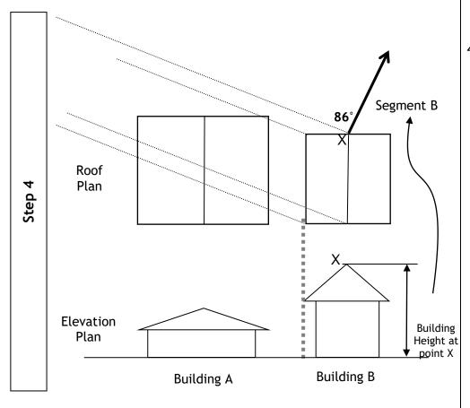
4. Choose one edge on the roof plan of Building B to draw the altitude angle. For this illustration, point X was used, but any roof edge may be used successfully. Draw a line segment ("Segment B") at an 86° angle to the shadow line at Point X (this will be parallel to the AM angle). The length of Segment B should be equal to the building height at point X, where Segment B is drawn.
