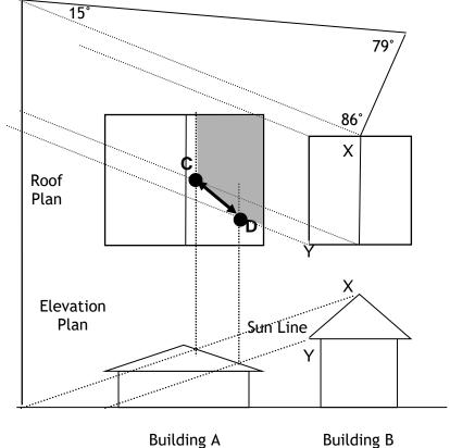
11. Locate where the two sets of the lines intersect on the roof plan of Building A. Shade in the corresponding amount of shadow on the roof plan. The diagonal line was drawn between points C and D to reflect the shadow of the roof form between the top of the ridge and the lower edge of the roof.
