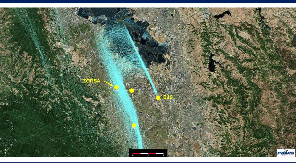
Tracks through 1 NM radius circle around ZORSA = 502 (45.2%) Average Altitude passing ZORSA = 2,730 feet MSL
