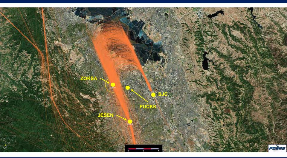
Tracks through 1 NM radius circle around ZORSA = 1,196 (75.3%) Average Altitude passing ZORSA = 3,040 feet MSL
