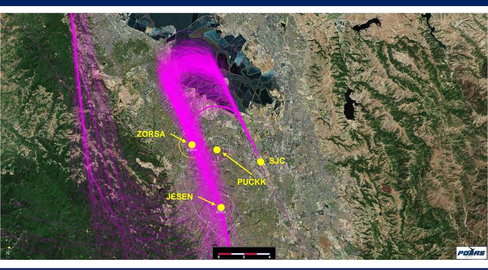
Tracks through 1 NM radius circle around ZORSA = 1,043 (82.6%) Average Altitude passing ZORSA = 3,080 feet MSL
