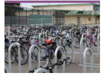
Bicycle parking can be designed for short-term or long-term use and includes bicycle racks (pictured), bicycle cages, lockers, and bicycle stations, among other designs. Parking should allow for bicycles to be locked to the rack at two points of the bike frame, sufficiently spaced from each other, and in a secure, well-illuminated area.
