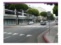
These markings, also referred to as "shark's teeth," are placed on the roadway 20-50 feet before a midblock crosswalk or crosswalk at an uncontrolled intersection to indicate where drivers should stop and wait for people to cross. These markings have been shown to increase driver yield compliance.
