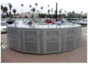
Bicycle lockers and secure parking areas are common long-term bicycling parking styles. Bicycle lockers vary in design and operation, ranging from keyed lockers that are rented to one individual on an annual or monthly basis to e-lockers that can be reserved in hourly increments and unlocked with a credit card or an access code.
