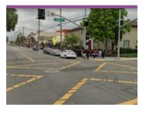
Traffic signals can be programmed to create a "pedestrian scramble" which shows red lights to vehicles in all directions, and allows people walking to cross the intersection in any direction.
