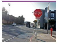
A stop sign is a traffic control device used to regulate traffic through an intersection. In general, the implementation of stop control is regulated by the Federal Highway Administration and requires a technical analysis be conducted before a stop sign can be installed.
