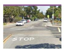
Stop lines are solid white lines that extend across approach lanes. They may be used to indicate the point behind which vehicles are required to stop in compliance with a stop sign, or another traffic control device that requires vehicles to stop.
